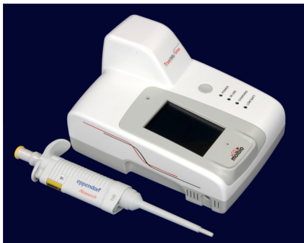
Fig. 1 – TrueNAT micro PCR device for chip-based real-time PCR.
