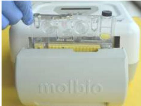
Figure 9: Cartridge being placed in cartridge holder
