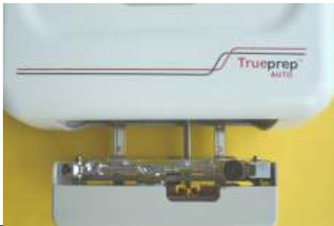
Figure 10: Cartridge placed in cartridge holder in correct orientation
