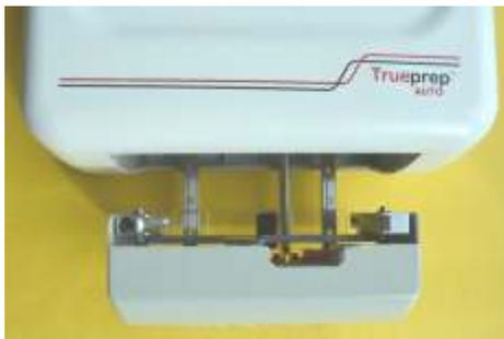
Figure 8: The cartridge holder opened after eject button is pressed
