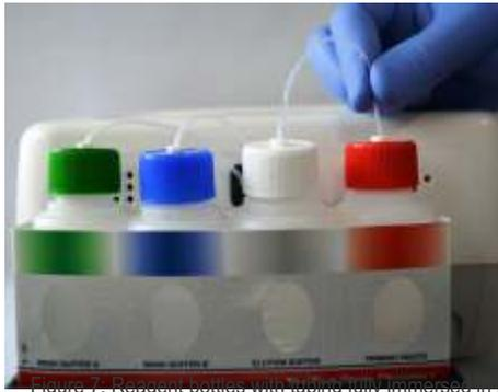
Figure 7: Reagent bottles with tubing fully immersed in liquid
