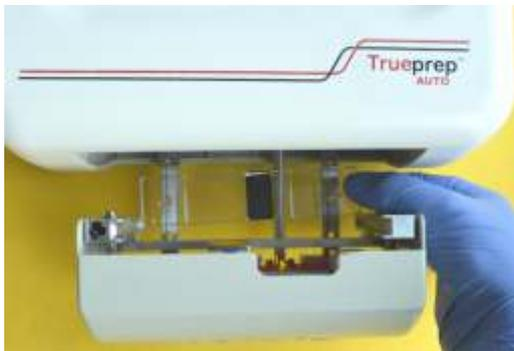
Figure 12: Tray removal from cartridge holder
