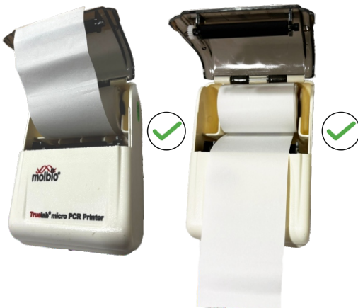
Figure 2: Right way to feed 75 GSM Paper.
