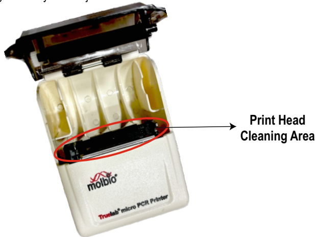
Figure 4: Procedure to clean the printer head
