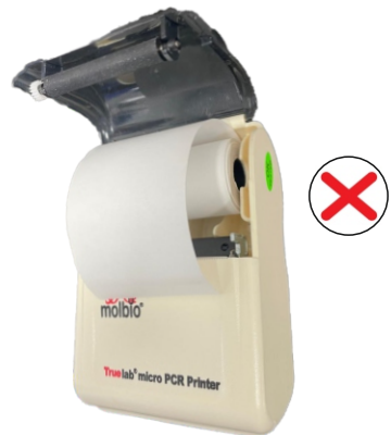
Figure 3: Wrong way to feed 75 GSM Paper.
