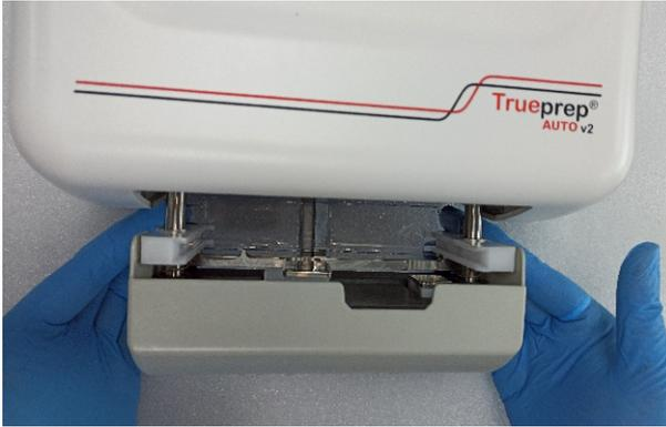
Figure 15: Replacement of discarded Replaceable tray with new
