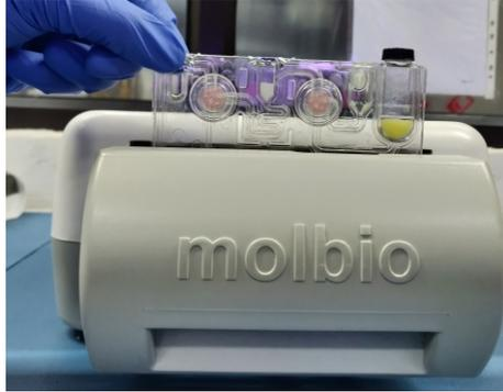
Figure 11: Cartridge being placed in cartridge holder
