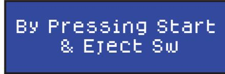
Press Start and Eject button together, buffer count will reset to zero and following will be displayed.
