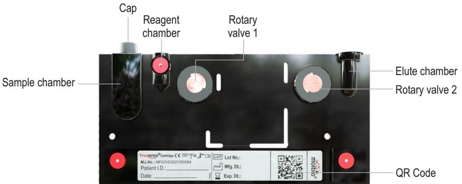
Figure 3: Disposable Trueprep® **AUTO** cartridge for sample processing
