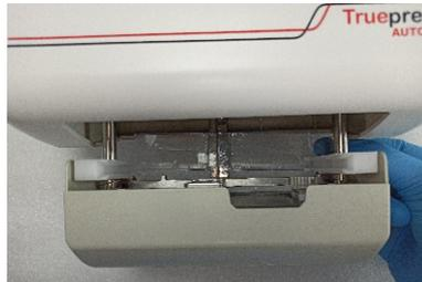
Figure 14: Removal of Replaceable Tray from cartridge holder
